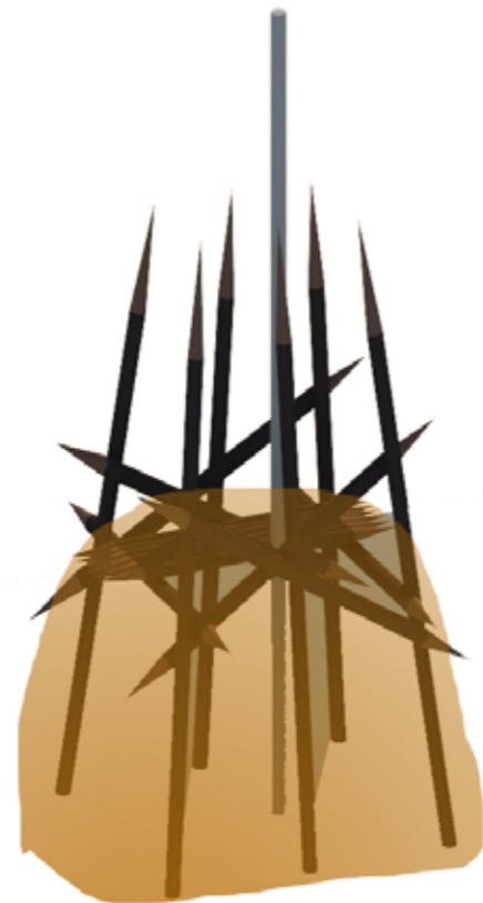
2. Stabilizing crafters connects the primary poles . Horizontal joists are placed as a mezzanine floor for hen coop. More hay is then added.
